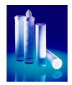
TOPLIFE TPR is manufactured with polypropylene. The filter media is obtained by winding around the internal core several polypropylene layers, having different porosity and permeability from external to internal; the outer section retains larger particles while the inner section provides filtration rating with efficiency of 99,98%. The different consistency of the layers allows to manufacture cartridges with filtration ratings larger than 10 microns.
